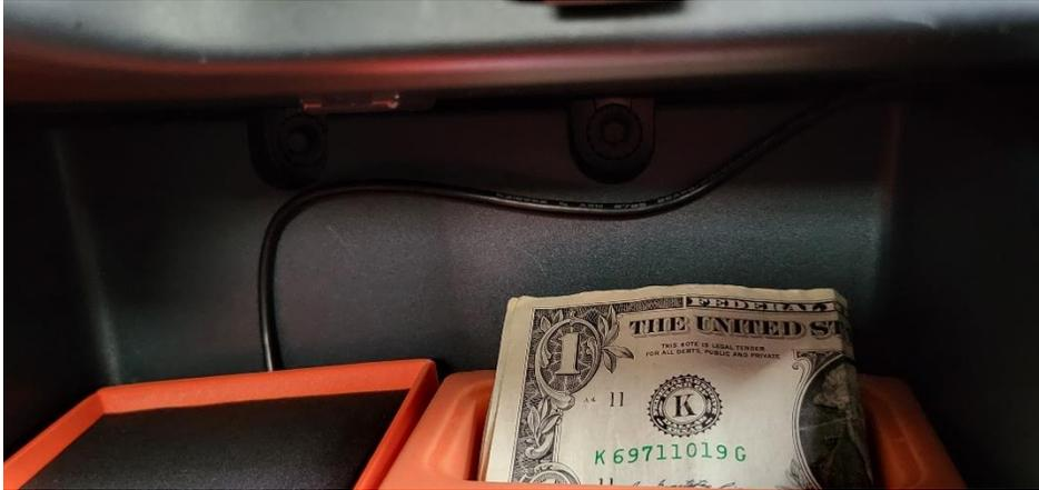
4) Plug in Type-C cable to wireless pad, and install charging pad into cubby pocket
