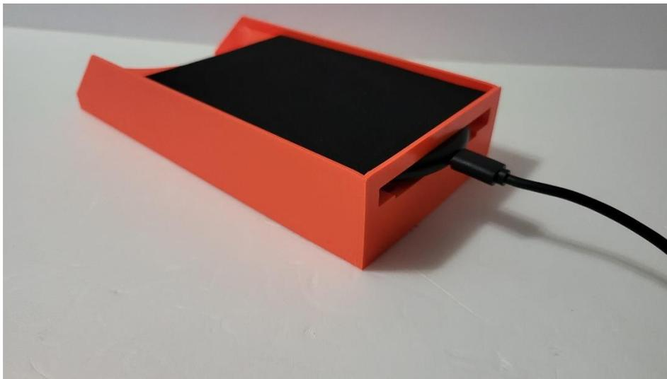
5) Adjust wireless pad for perfect fitment by sliding it forward or backward for proper alignment for charging
