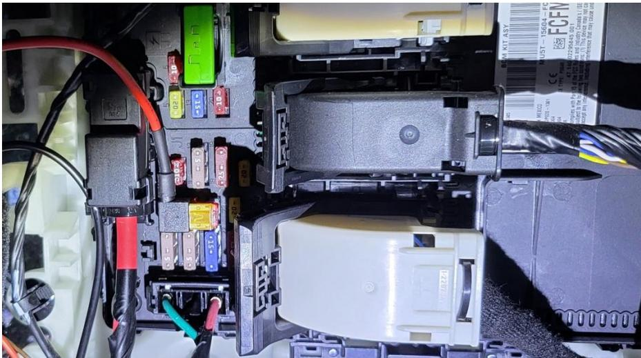
3) Using 10mm driver, loosen bolt as shown and attach ground wire here
