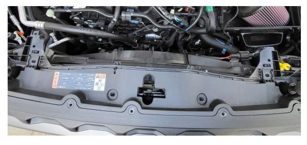
4. While carefully pulling grill assembly forward, release the lock tabs to partially disassemble
