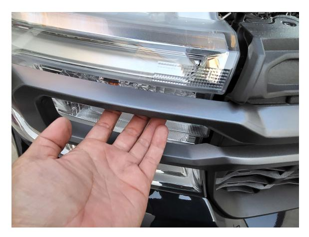
5. Now with the top portion of the grill released, you will have enough slack to route the wires underneath the top of the grill area, leading your LED wires to where your LED wires will be installed. Ensure that your wires are routed in the gap of the top area of the underside of the grill. There is also the entry ducting for the intake piping underneath this area to be mindful of.
