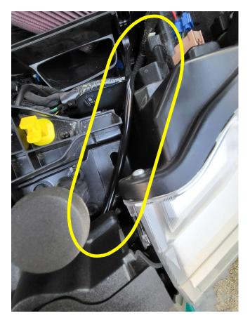
6. Insert LED light assembly into grill, plugging in each light to the harness.
