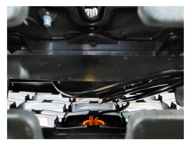
Route the wire in between the opening of the side of the headlight and the grill
