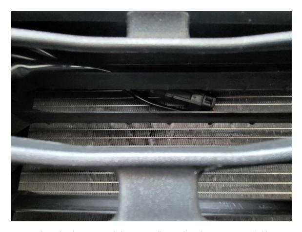
8. Using the updated wire taps and pliers - you will crimp the red positive wire to the blue wire behind the turn signal bulb connector. Use the pliers to carefully crimp and lock into place the black wire to the black negative wire at the connector.
