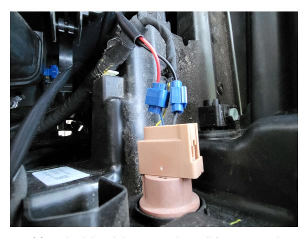
Verify function by unlocking or locking your Maverick. Reinstall all parts in reverse order, tucking excess wire in safe areas of the engine bay.
