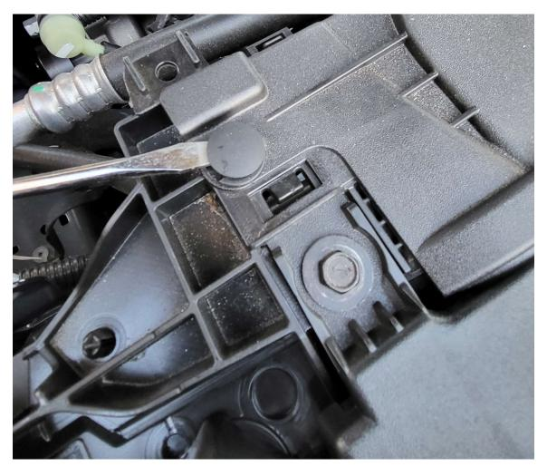
3. Remove cold air ducting by pulling up
