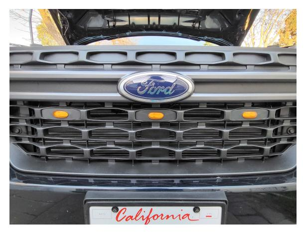
7. Once all LEDs are plugged in, you can tuck the wiring on top of the most upper fin behind the grill
