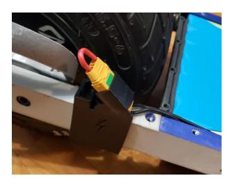
Step 12: Reconnecting main harness and installing voltmeter
