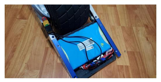
Step 10: seal switch wires exiting/entering battery box
